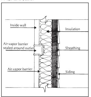
sation can occur causing water or frost damage, which leads to the growth of mold or mildew. Rooms shut off from heating sources or used only intermittently, such as bedrooms or closets, can be problem areas, as can areas made cold by drafts or spaces behind furniture on outside walls. Uninsulated walls and windows, and wall, ceiling or floor areas where insulation is missing or has shifted, such as the junction where wall meets ceiling, are other key locations (Figure 2).
