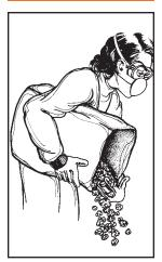
Figure 2: Wear protective clothing when installing insulation.
